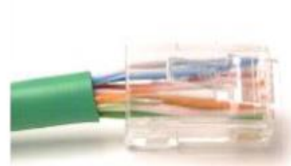
Poorly terminated UTP cable
